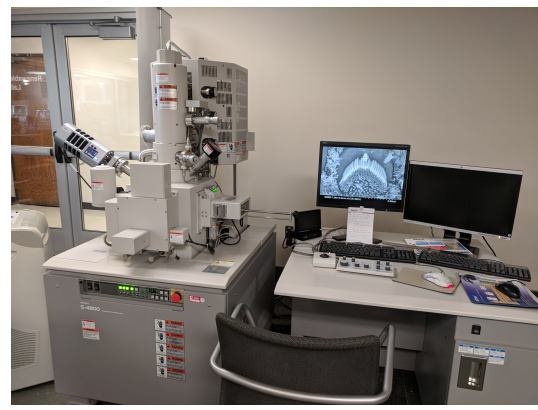
(b) Hitachi S-4800 Field Emission SEM with Energy Dispersive X-ray Spectroscopy
