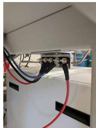
(c) Connections going into the glovebox to the electrochemical cell
