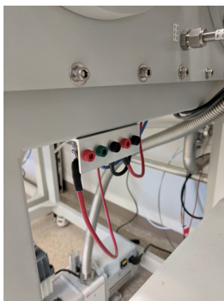
(b) Connections for the potentiostat
