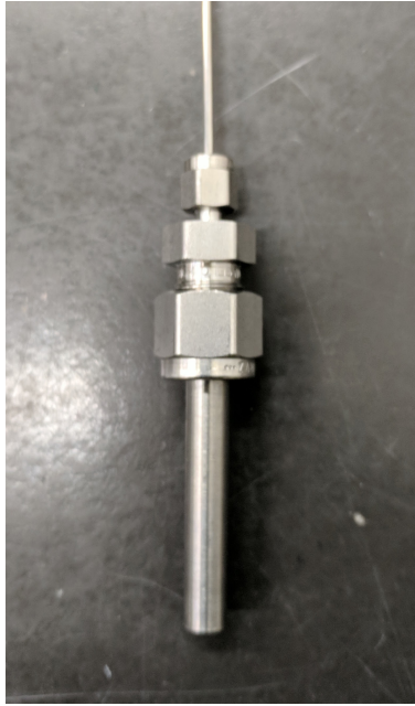
Figure 5.5: Photograph of Tb rod anode secured in a custom Swagelok
