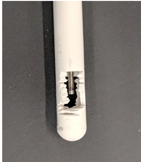
Figure 5.11: Photograph of custom mullite tube basket
