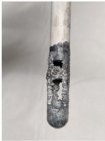
(a) Frozen salt and metal deposit on mullite tube
