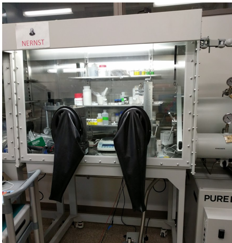
Figure 5.1: Photograph of glovebox used for electrochemical tests
